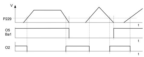
To avoid O2 continuously switching over during nominal speed value disturbance (during synchronization applications), a minimum pulse time (≡ minimum positioning time) is defined.
